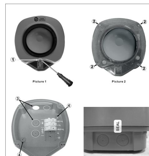
NOTE!!! After finishing the installation place the sticker SEAL as shown in the picture above.
