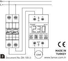
Setting the high voltage value; Press the Up Button for 1 second to set the high voltage value. The program led will start flashing and the high voltage value stored in the device will be displayed on the screen. While the high voltage value is displayed on the screen, the desired value is adjusted by using the Up/Down buttons. The set value is saved by pressing the SET button. The program led will turns off and the input (mains) voltage value will be displayed on the screen.
